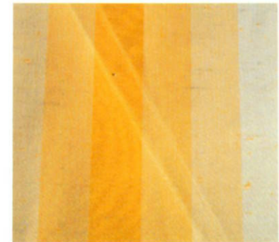
Knickfalten Creasemarks of a width of material
